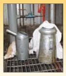
Open top, unsealed homemade containers deliver contaminated lubricants into the heart of your machinery.
